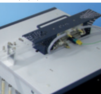
Large diameter (Ø 30 mm) for typically 1-inch samples like used in AWS A4.3
